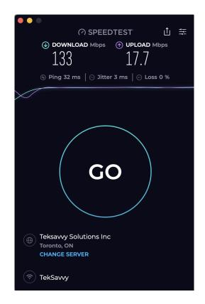
So the upload number on the top right is the important value (17.7 Mbps above). If you are using a dedicated hotspot, this may involve moving to different points in the rink to get a better signal. It's possible to site the hotspot up to about 50m away from the Mac and still maintain a good signal, provided you have a line of sight to the MiFi (no walls in the way). This flexibility allows for searching
